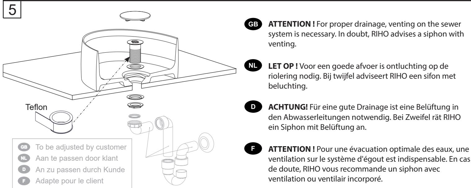
**GB** **ATTENTION !** For proper drainage, venting on the sewer system is necessary. In doubt, RIHO advises a siphon with venting.
